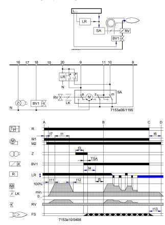
Load control with a 2-position controller. During burner off times, the air damper is closed.
