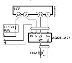
Measurement made on the flame detector
