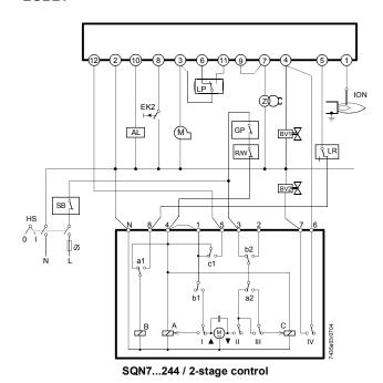
Burner without fan and without air pressure switch (LP)
