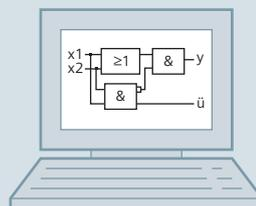
Complex local control tasks can be easily realized using programmable logic control (PLC) functions. The integrated, freely programmable logical function blocks reduce the need for additional external controls. No other investments are required – even for challenging applications.
